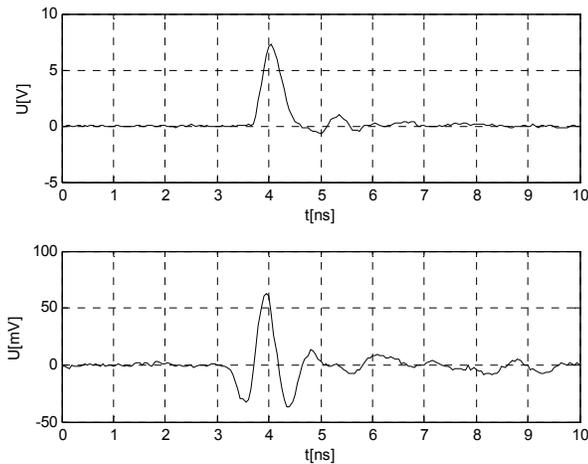
Fig. 5. Top: measured positive pulse via cable directly connected to oscilloscope. Bottom: transmitted pulse via antennas in an anechoic chamber.
