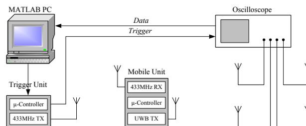
Fig. 1. Architecture of the low-cost experimental UWB positioning system.
