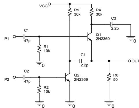
Fig. 4. Circuit diagram of the bi-phase pulse generator using the avalanche effect of two NPN-transistors.
