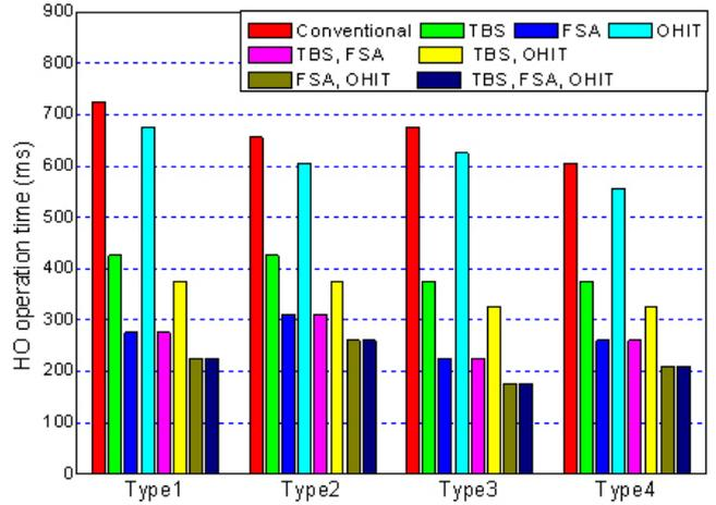
Fig. 7. HO operation time analysis (cell-loading 0%).
