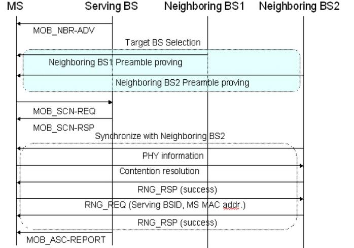
Fig. 5. Proposed Network Topology Acquisition.
