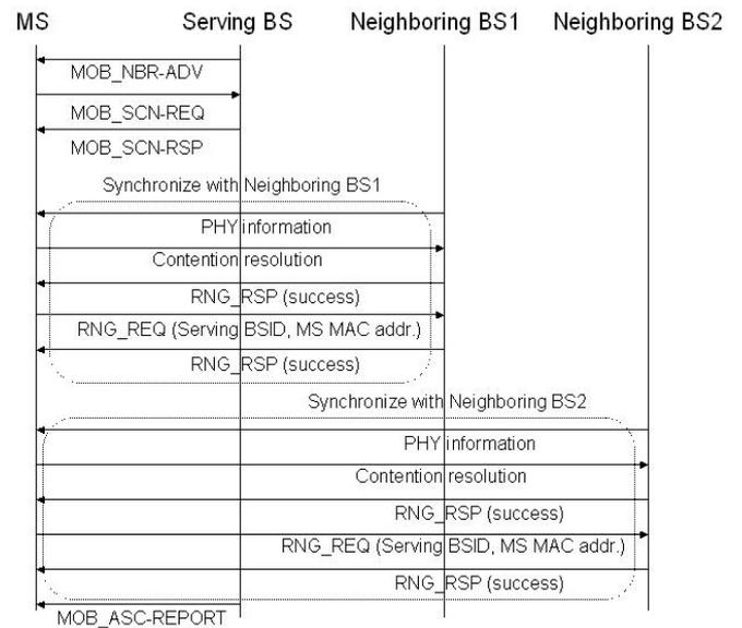
Fig. 2. Network topology acquisition.
