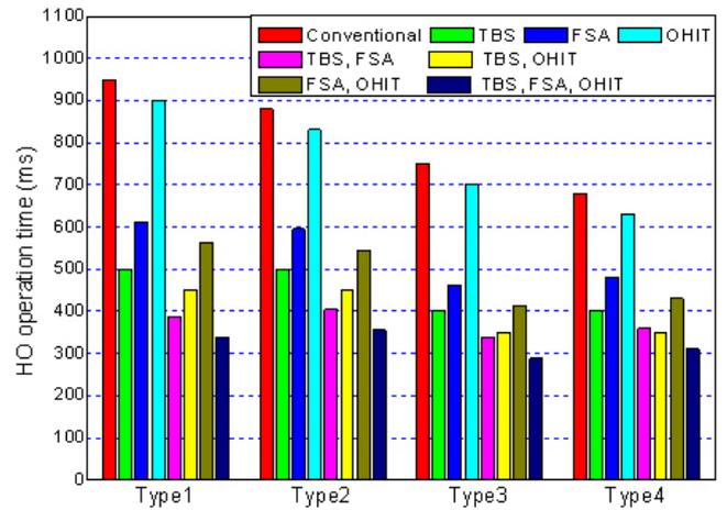
Fig. 8. HO operation time analysis (cell-loading 50%).
