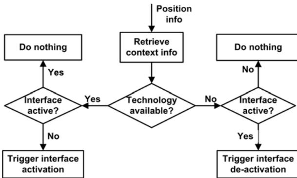
Figure 5. Interface activation or deactivation algorithm
