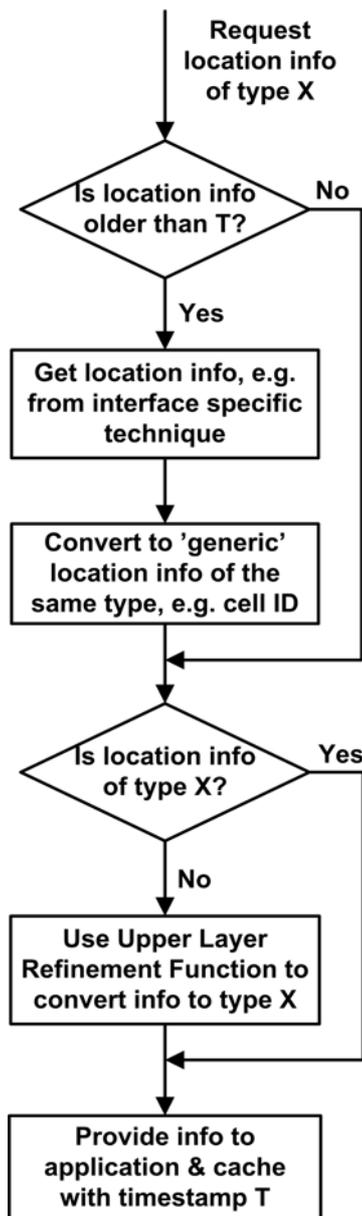
Figure 3. The Positioning Function Coordination Algorithm
