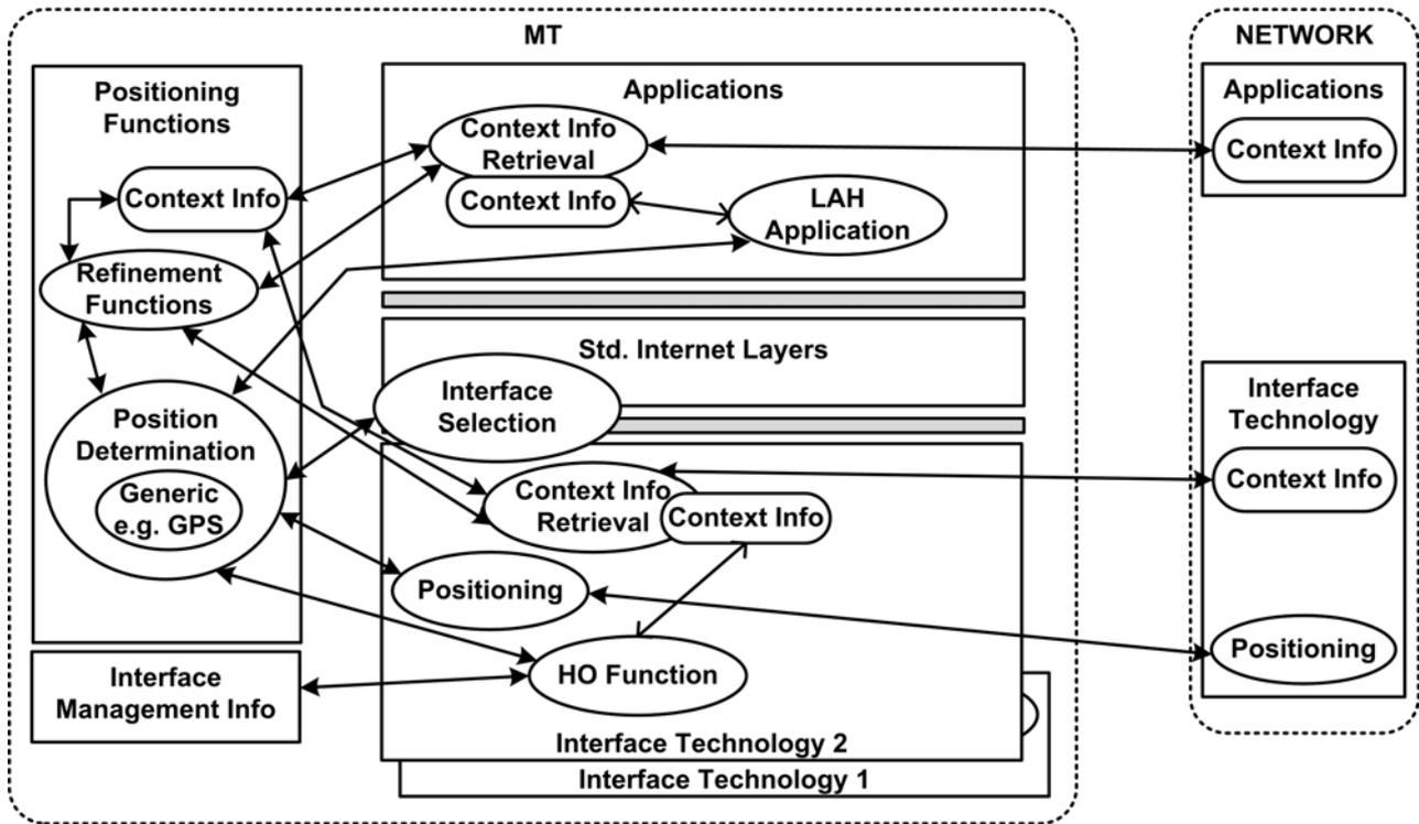
Figure 2. Multimode mobile terminal architecture for LAH
