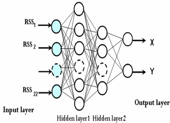
**Fig.6 NN architecture used for this positioning issue**
