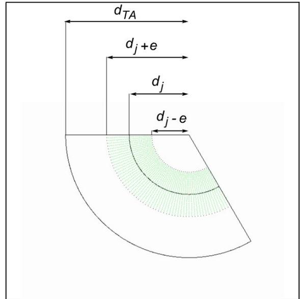
Fig. 5. Exploiting equation (4) to further specify the area in which we search for MS location candidates
