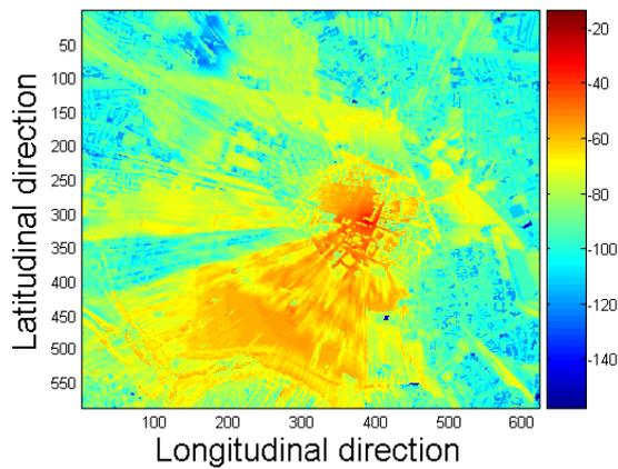
Fig. 2. Map of RxLev (dBm) generated by the radio wave propagation prediction tool for a base station antenna. The simulation is performed over an area of approx. 9 km<sup>2</sup> divided into pixels (621 x 588 pixels in the longitudinal and latitudinal directions respectively) with a resolution of 5 m
