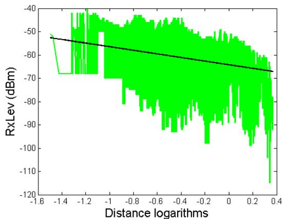
Fig. 4. Relationship between the received signal strength and logarithm of distance to serving antenna for an example cell using the prediction database and the LS linear model
