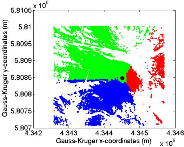
Fig. 1. Results of the preprocessing step for a sectorized cell where the pixels (locations) served by each sector antenna are depicted in different color. The black dot represents the BS location.
