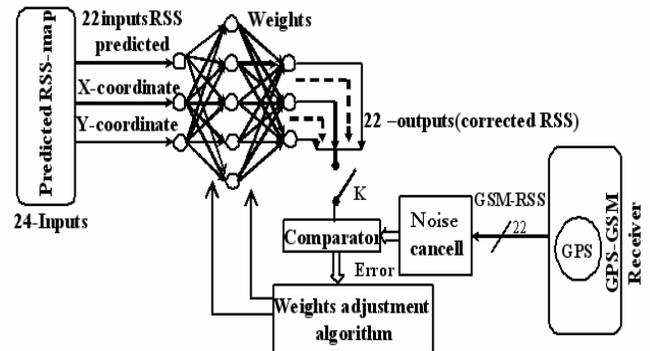
Figure 4: Block diagram used for calibration
