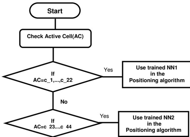
Figure 3: Flowchart showing the NN to be used in the positioning algorithm
