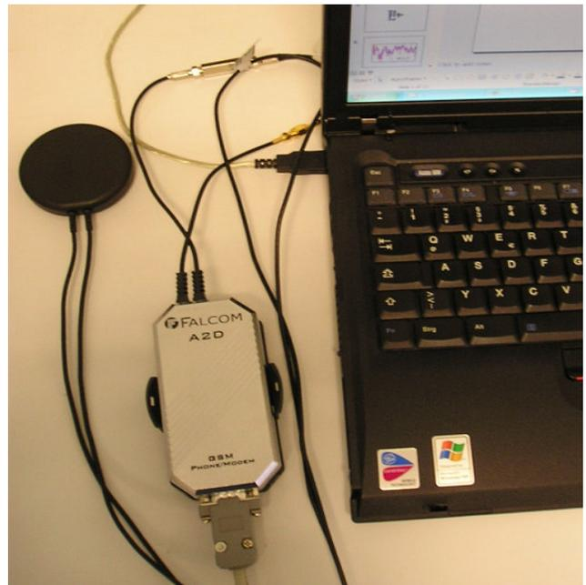
Figure 5: GSM-GPS antenna and modem. Used for RSS collection
