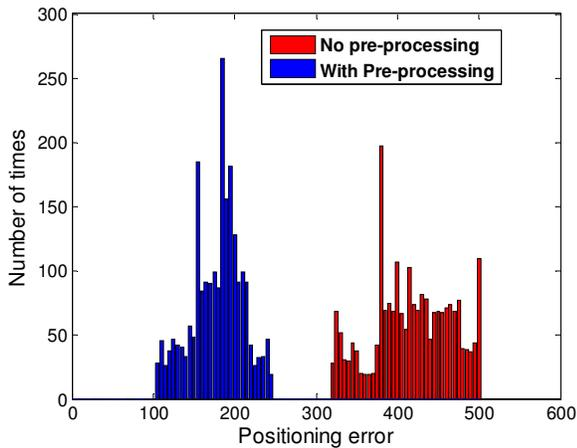
Figure 10: Histogram \_Root of mean squared positioning error in meter.
