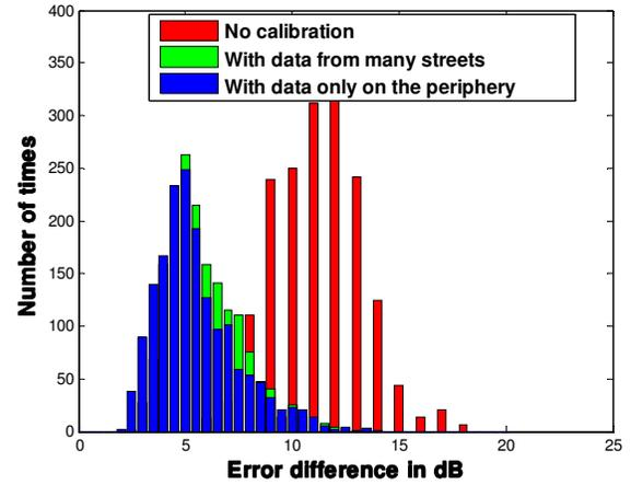
Figure 6: Histogram showing the dependence of calibration error on different scenarios
