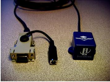
Fig. 4. InertiaCube (IMU)
