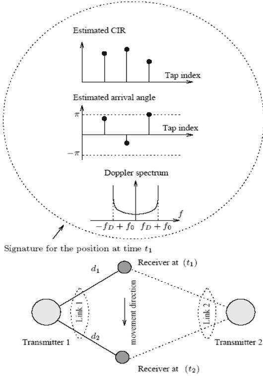
Figure 1: position determination based on the estimated channel [2]
