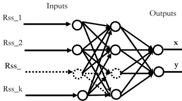
Figure 1. NN architecture for function approximation
