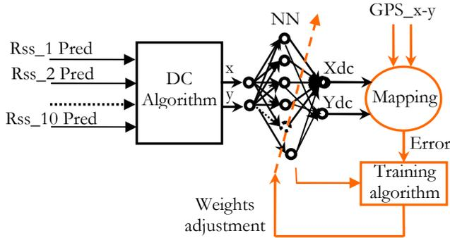
Figure 8. Block diagram of the DC positioning correction
