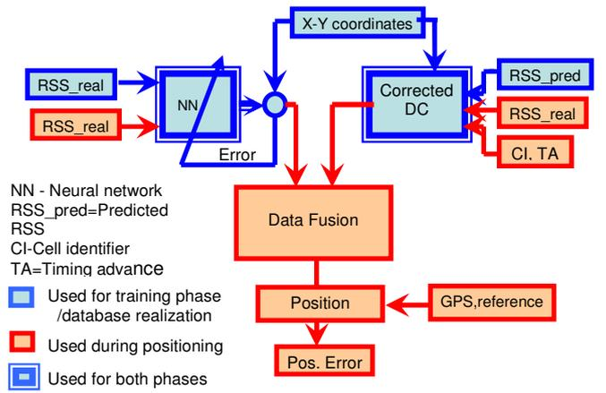
Figure 9. Block diagram of the fusion process
