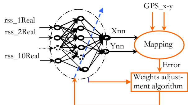
Figure .3. NN training and positioning block diagram (In the NN positioning phase, only black colored part of the figure is used).
