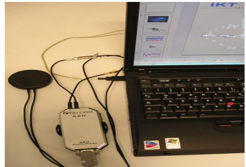
Figure 10. GSM-GPS antenna and Modem used
