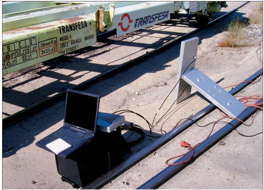
Figure 3. Our test setup, showing RFID equipment for range measurements, using 2.5 cm × 2.5 cm tags on moving targets.
