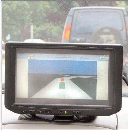
**Figure 1.** TrafficView's near-view panel displays cars as green or red rectangles, depending on their speed relative to the current car. In the picture, the car in front of the SUV brakes and becomes red in the panel.
