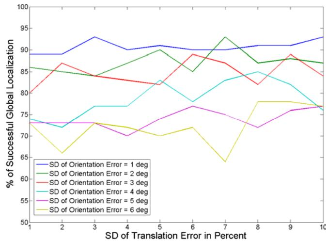
Figure 9: Percentage of successful global localization with varying standard deviations of IMU translation and orientation.
