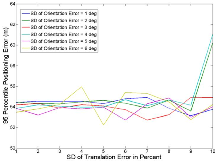
Figure 8: 95 percentile position tracking error.
