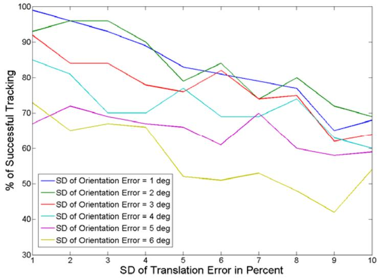
Figure 5: Percentage of successful position tracking with varying standard deviations of IMU translation and orientation.
