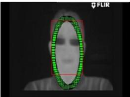
Figure 6. Output of face detection algorithm.
