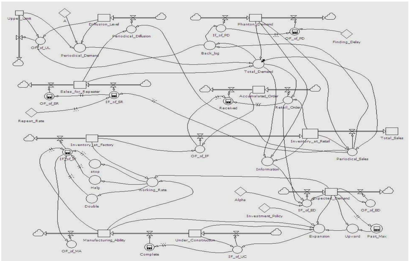
Figure 10. State flow diagram of Tamagotchi™ Supply chain model
