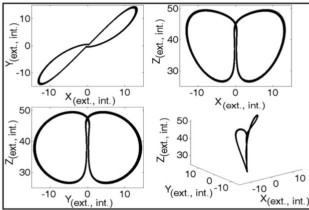
Figure 6. Alleviation of the chaotic effect caused by external perturbation with adaptive synchronization
