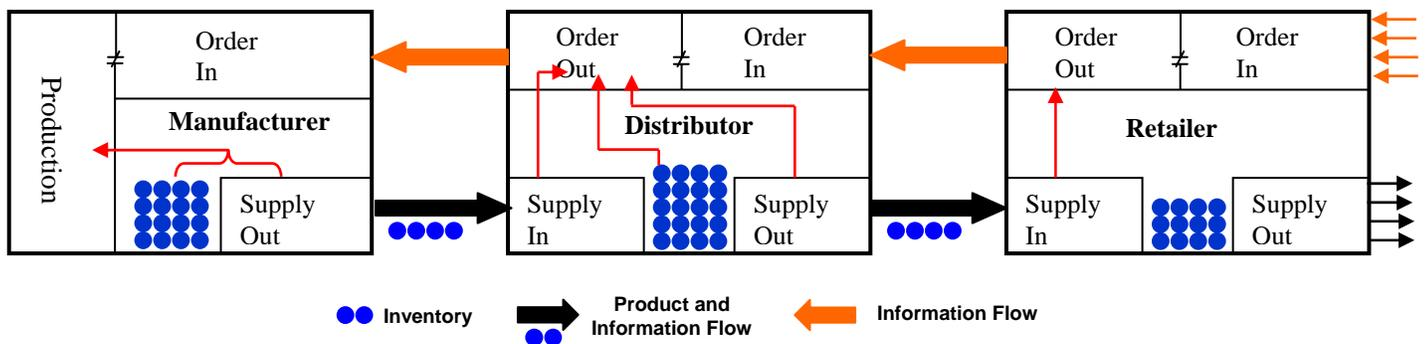
Figure 2. Model of a three echelon supply chain
