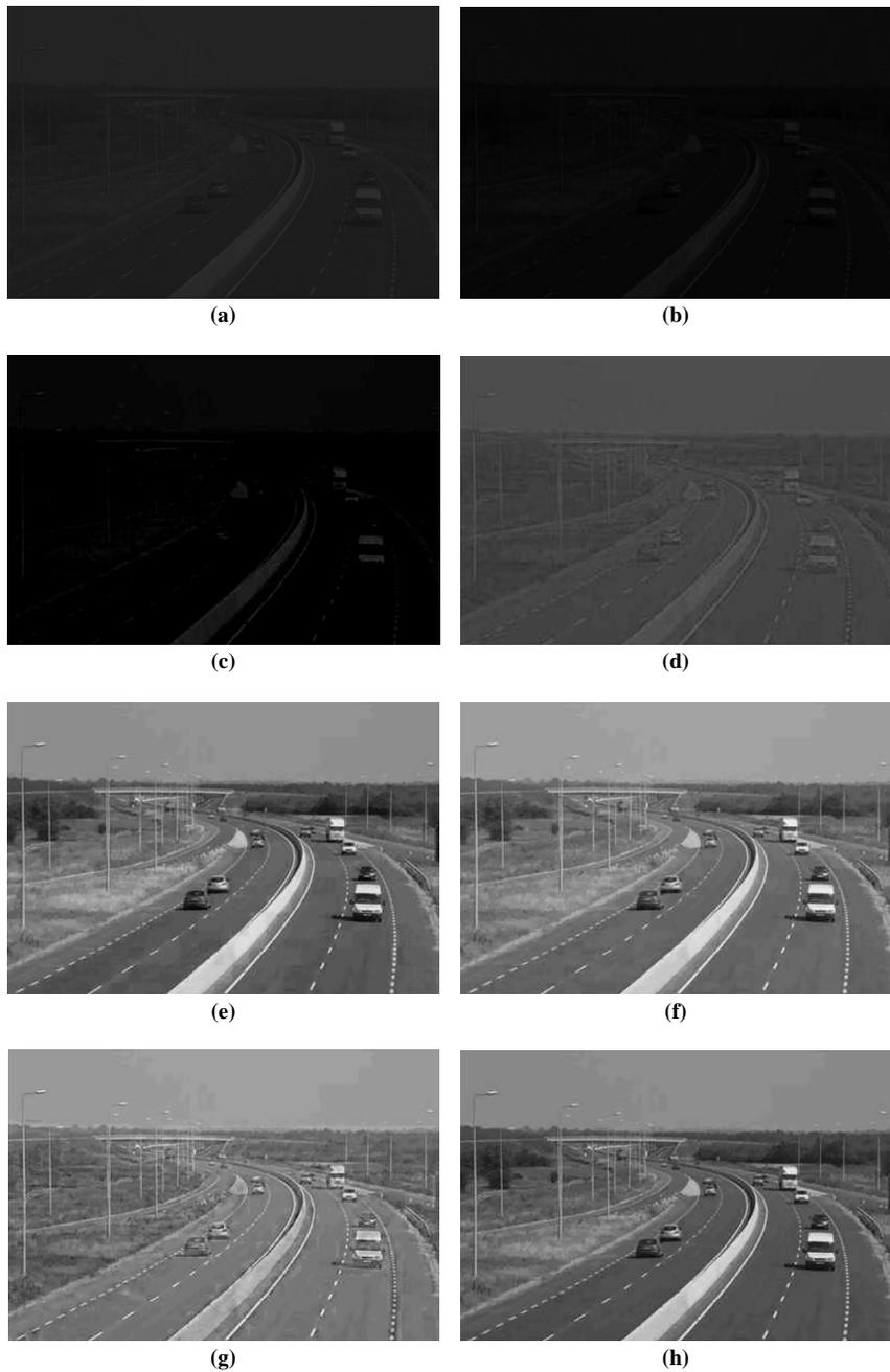
**Figure 8.** (a) Input image, (b) original R-channel, (c) original G-channel, (d) original B-channel, (e) improved R-channel, (f) improved G-channel, (g) improved B-channel, (h) output image by combining all the improved channels
