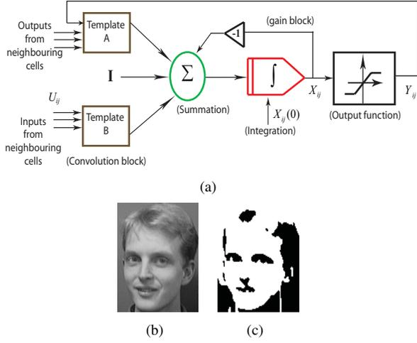
Fig. 3. (a) Schematic representation of the CNN (b) The input image (c) The genetic cellular neural network output image
