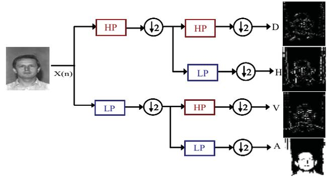
Fig. 2. Wavelet coefficients decomposition in discrete wavelet transform
