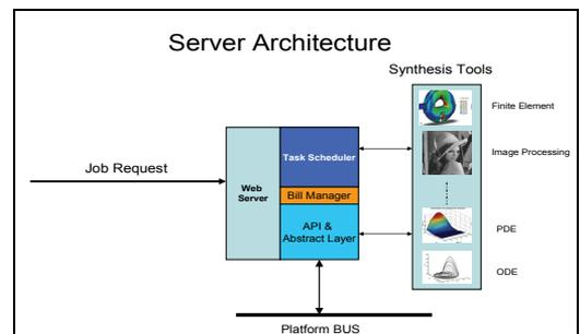
Figure 6. Core idea of the server architecture intended for the CNN based super-computing platform to enable real-time Computational Engineering. It is a detailed description of the central server given in Fig. 5.
