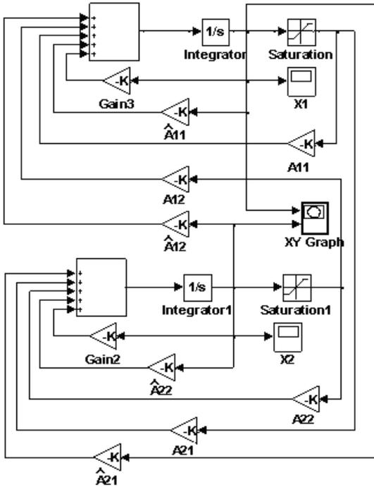
Figure 3. SIMULINK graphical representation of the CNN- computing platform to solve (3).
