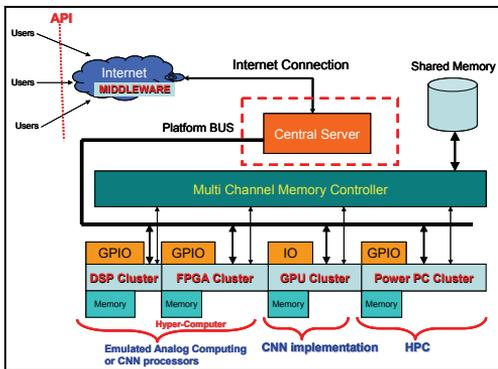
Figure 5. Global architecture of the computing platform planned to enable a real-time computational Engineering. Diverse users may access the CNN processor platforms in a remote way through the Internet
