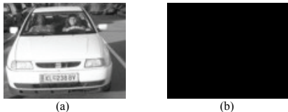
Figure 3: Result of the image processing in the case where the system is the critical equilibrium point P_c(0, 0, 0, 0) : input image (a) and result of the processing (b), leading to an output image which is completely dark (Quenching phenomenon).
