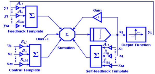
Fig. 1b: SIMULINK graphical representation of the basic model of a state-control CNN cell (SC-CNN) coupled to  $(M-1)$  Neighbours.
