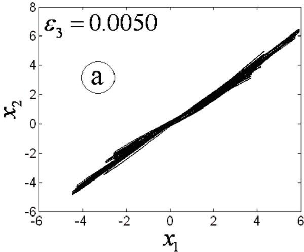
Fig. 4a. Direct numerical simulation results (Turbo-c) showing the projection of the regular attractors of the master and slave systems in the plans  $(x_1, x_2)$  for  $\epsilon_3 = 0.0050$ . This projection shows the regime of regular synchronization in the Master-slave-auxiliary coupled system. Same values of parameters as in Fig. 3a.
