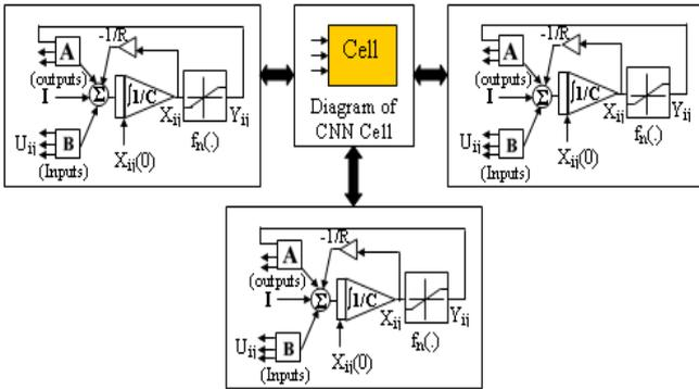
Fig. 2a: Schematic representation of the 3 CNN cells needed to implement each subsystem (i.e. master or slave or auxiliary) on top of SIMULINK.
