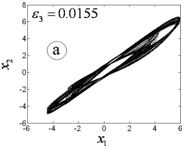
Fig. 4b. Direct numerical simulation results (Turbo-c) showing the projection of the chaotic attractors of the master and slave systems in the plans  $(x_1, x_2)$  for  $\epsilon_3 = 0.0155$ . This projection shows the regime of chaotic synchronization in the Master-slave-auxiliary coupled system. Same values of parameters as in Fig. 3b.
