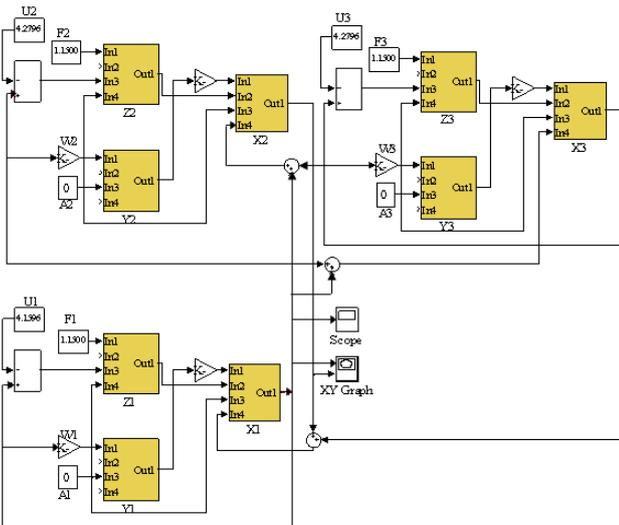
Fig. 2b: Schematic representation of the complete CNN-processor (master-slave-auxiliary) implemented on-top of SIMULINK.
