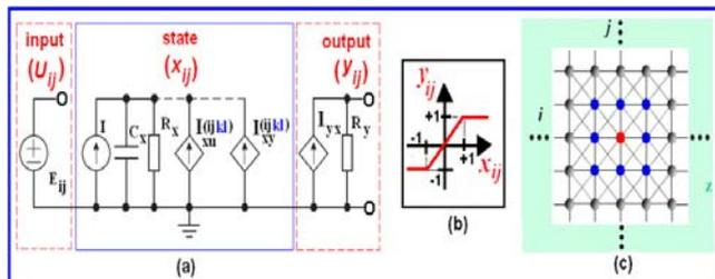
Fig. 1a: (a) The basic CNN cell defined as a nonlinear first order circuit, (b) The PWL sigmoid function, and (c) A CNN architecture composed by a two-dimensional array of  $M \times N$  cells arranged in a
