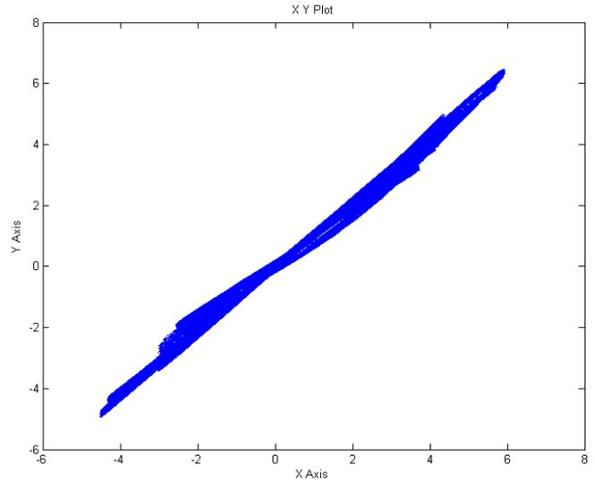
Fig. 3a. Simulation results using CNN on top of SIMULINK showing the projection of the regular attractors of the master and slave systems in the plane  $(x_1, x_2)$  for  $\varepsilon_3 = 0.0050$ . This projection shows the regime of regular synchronization in the master-slave-auxiliary coupled system. The other parameters are defined in the text.
