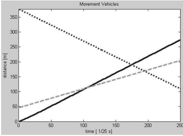
**Figure 2: Path-time diagram of an overtaking maneuver with an oncoming vehicle**
