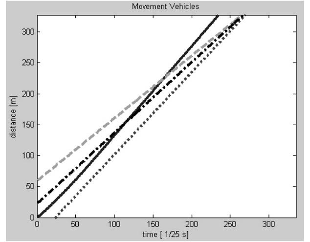
**Figure 3: Path-time diagram of an overtaking maneuver with an approaching vehicle and a vehicle in the overtaking lane**
