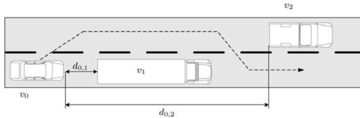
**Figure 3 Overtaking scenario involving three vehicles**
