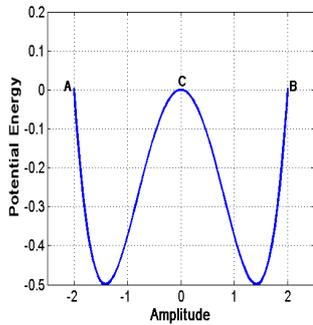
Fig. 1 The Duffing oscillator with two-well potential
