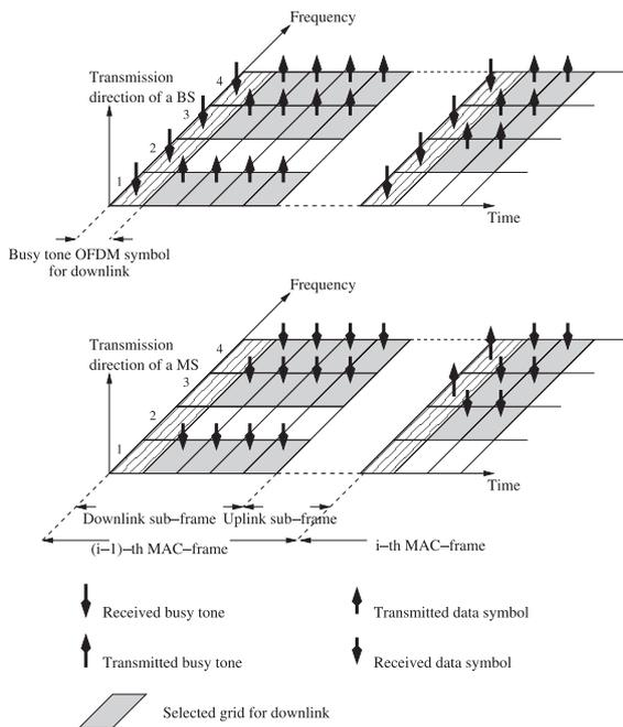
Fig. 3 MAC-Frame structure for the proposed algorithm.
