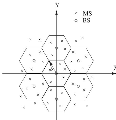
Fig. 5 Scenario for simulations of a cellular network.
