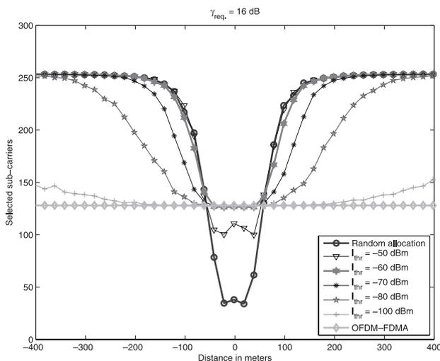
**Fig. 12** Number of selected sub-channels obtained by different allocation methods.
