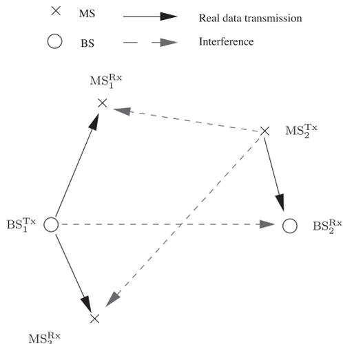
Fig. 1 Co-channel interference in OFDM/TDD networks with 100% frequency reuse.
