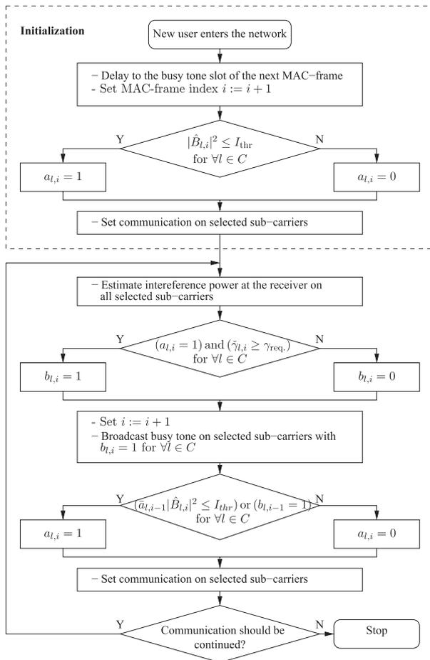
Fig. 4 Flow chart of the proposed DSA algorithm.
