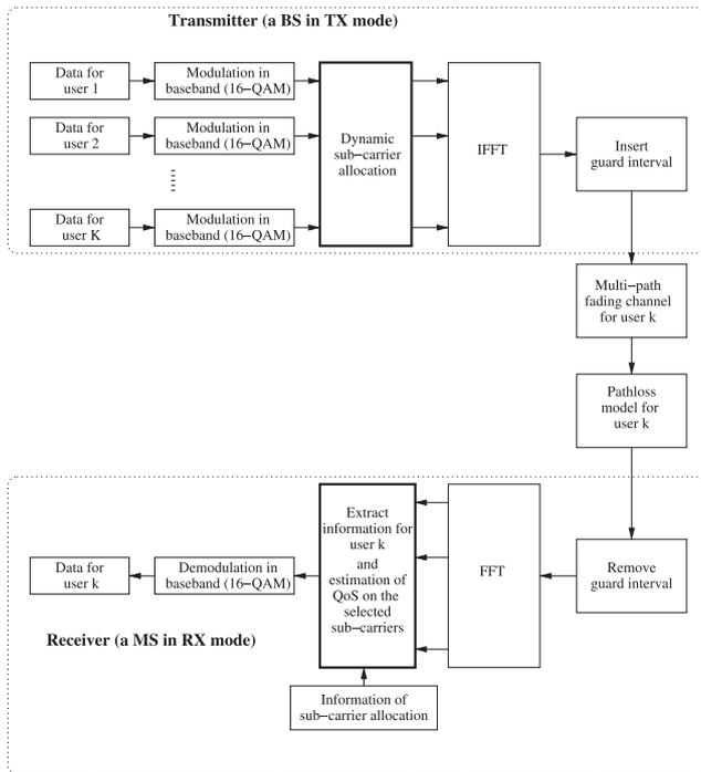
Fig. 6 A simplified model for downlink communication.
