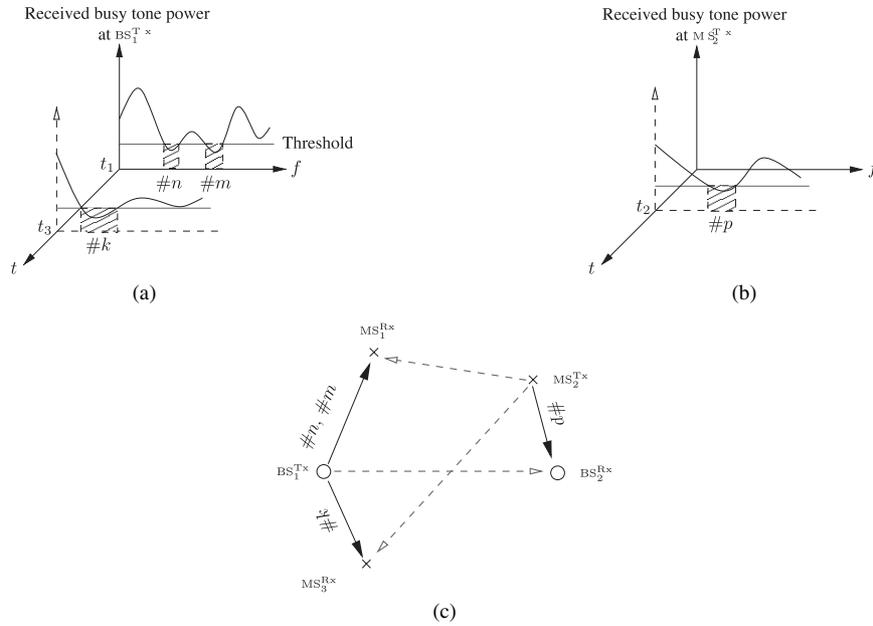
Fig. 2 Concept of the decentralized DCA for OFDM/TDD networks with 100% frequency reuse.
