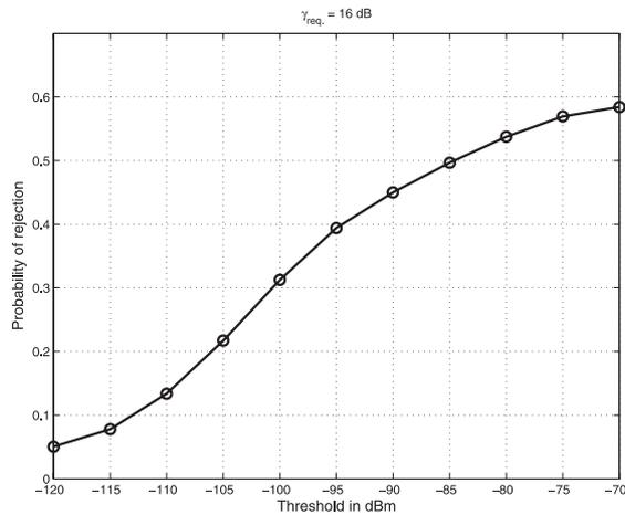
**Fig. 8** Probability of data rejection at receiver versus threshold.
