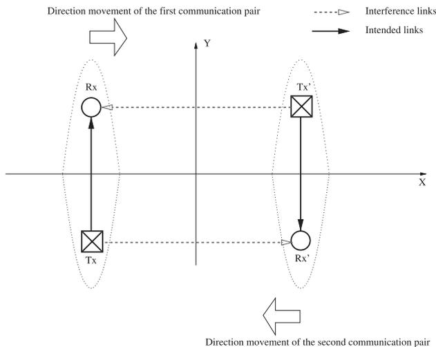
**Fig. 11** Simplification of the simulated adhoc scenario.
