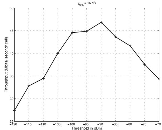
Fig. 7 Throughput of the system versus threshold.
