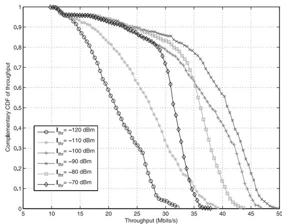
**Fig. 9** Complementary CDF of throughput obtained by proposed MAC for different levels of threshold.
